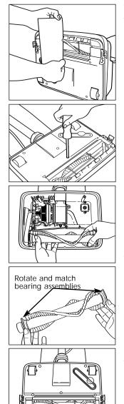
IMPORTANT: Unless the brush is worn as indicated above, both bearings must be in the "NEW" position. When rotating, both bearings must be in the "OLD" position. Unmatched settings will cause damage to your machine. To determine if the brush is worn, place a firm straight edge across the nozzle opening. If brush bristles do not extend beyond baseplate, brush should be adjusted.
